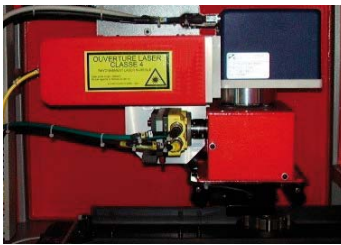
Integrated vision system (mark verification)
